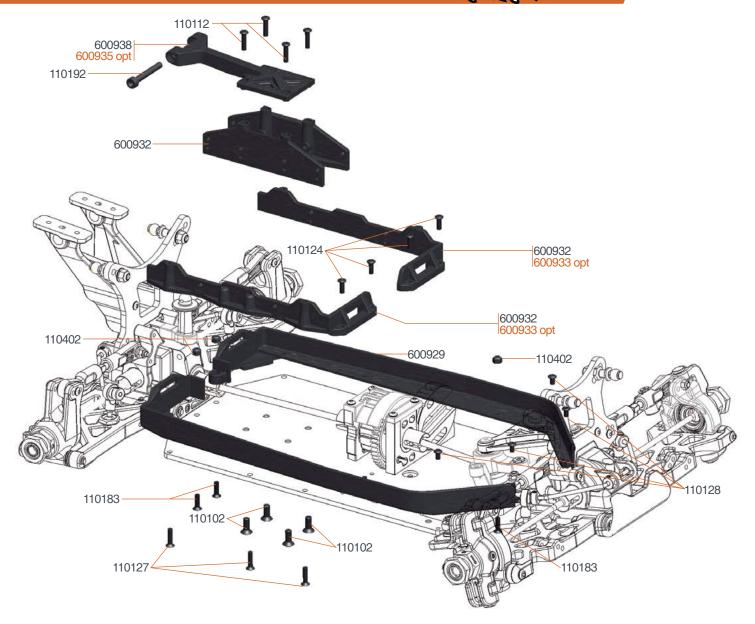
600933 Battery mount set block layout SRX8E 600935 Chassis brace / gear cover block layout (2) SRX8E
