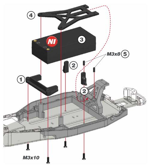
For being able to use the inline shorty battery configuration, right and left sideguards must be modified as show in the right picture. It is needed to cut 23.5mm of each wall shown in red in the picture.
