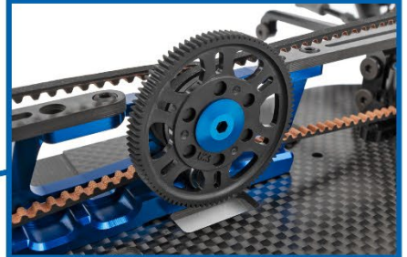
Mid-Motor Configuration with Symmetrical Belts
