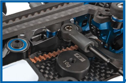
Floating One-Piece Servo and Bell Crank Mount
